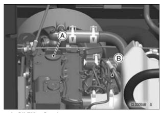
A. Oil Filler Cap 1 B. Oil Filler Cap 2
