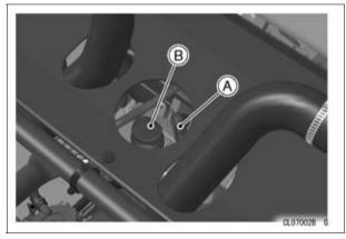
A. Spark Plug Cap B. Engine Oil Dipstick Cap
