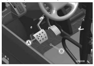
A. Brake Pedal B. Floorboard
