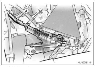
A. Throttle Cable B. Mounting Nuts
