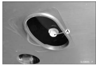
A. Engine Oil Drain Bolt and Gasket
