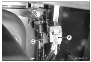
A. Fuse Box 2 B. Fuse Box 3 Lid C. Fuse Box 3
