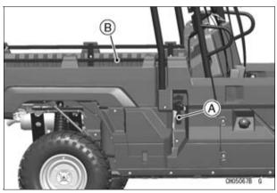
A. Cargo Bed Latch (Locked Position)
