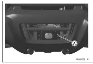
A. Winch-installing position
