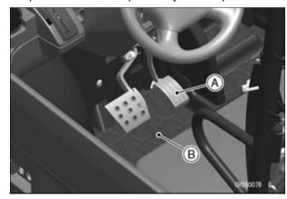
A. Throttle Pedal B. Floorboard
