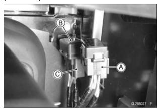
A. Fuse Box 2 B. Fuse Box 3 Lid C. Fuse Box 3
