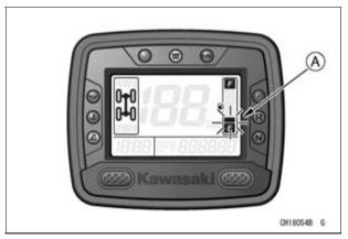
A. Blinking to warn of a low fuel level
