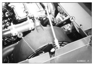
A. Cooling Fan Belt B. Cooling Fan
