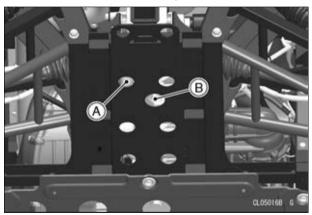
A. Transmission Case B. Oil Drain Bolt and Gasket
