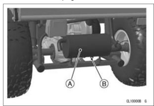
A. Spark Arrester (inside the muffler)
