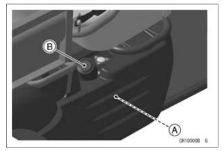
A. Fuel Tank B. Filling Cap
