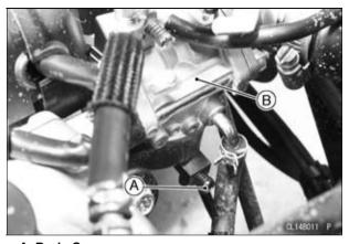
A. Drain Screw B. Carburetor
