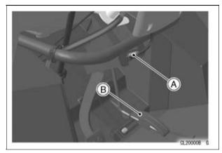
A. Brake Light Switch B. Throttle Pedal
