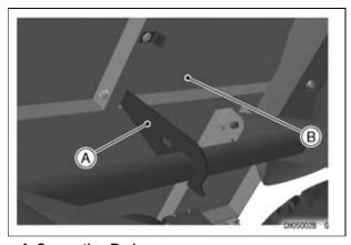
A. Supporting Rod B. Cargo Bed Bottom (Tilted Condition)
