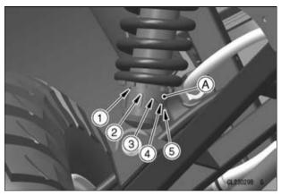
A. Spring Adjusting Sleeve (Turn with a hook wrench)
