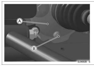
A. Front Final Gear Case B. Drain Plug
