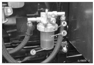
A.Water Separator B. Filter Element C. Float Ring
