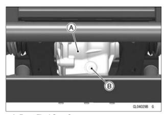
A. Front Final Gear Case B. Oil Filler Cap and O-ring
