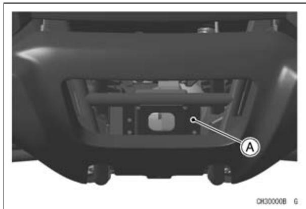
**A. Winch-installing position**
