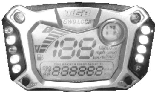
2. To change EPS mode, press the RESET button, the EPS system will toggle to the other available mode, which engage or disengage, “MIN” or “MAX”.
