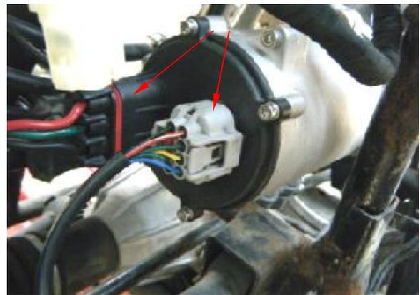
Remove the three mounting bolts ① of EPS body.
