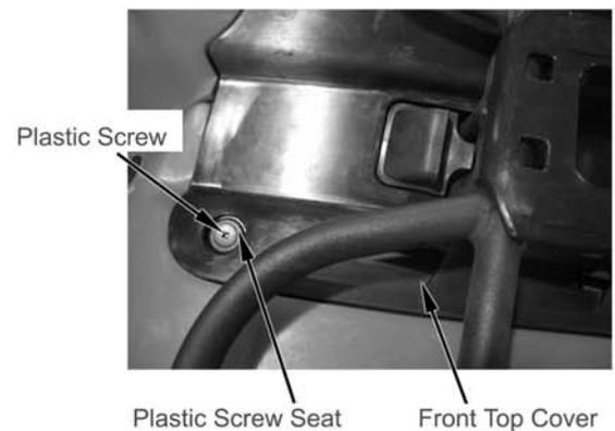
Separate clasps of top cover from fuel tank and front fender as illustrated on the right;
