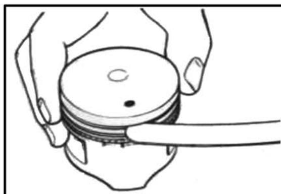
**Standard width of piston ring groove**
