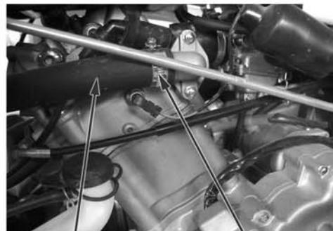
Water Outlet Hose, Engine    Clamp
