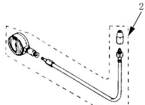
**Inspection of Oil Pressure****Oil Pressure: 130~170kpa at 3000r/min**
