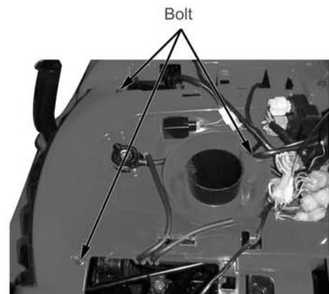
Remove 6 screws and nuts from left and right
