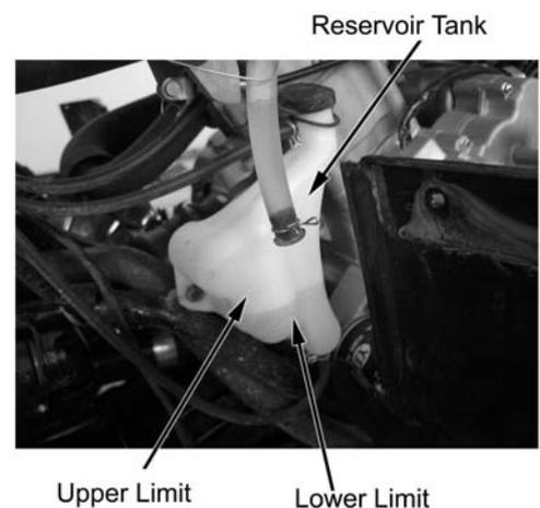
When the coolant level is below the LOWER limit, remove reservoir tank cap and add coolant till upper limit. (Add coolant or diluted original liquid).
