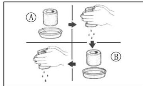
Inspect the filter element for tears. torn element must be replaced.
