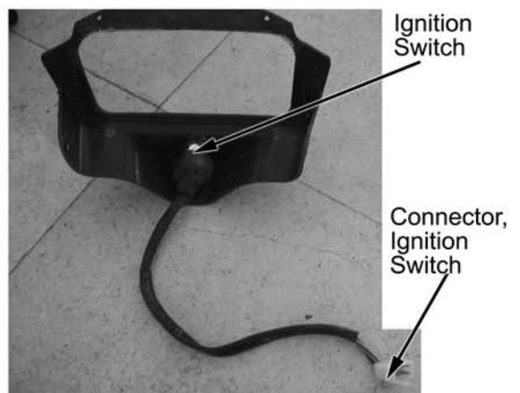
Check according to the following table if the connector terminals are in continuity.
