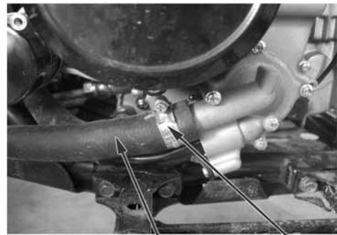
Water Inlet Hose, Engine    Clamp
