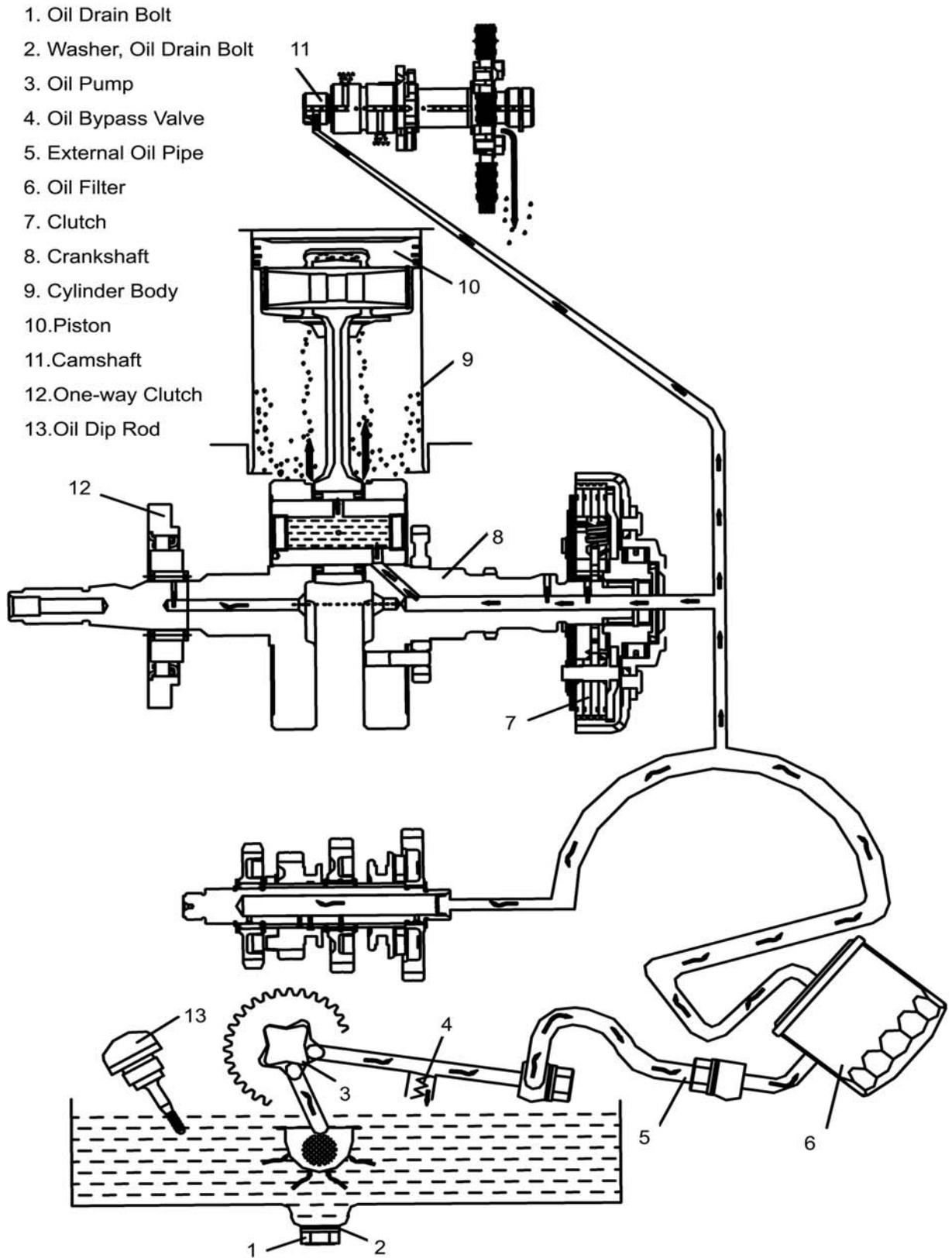
**Inspection of Lubrication System (→11-8)**
