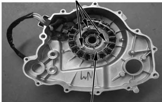
Stator, A/C Magneto
