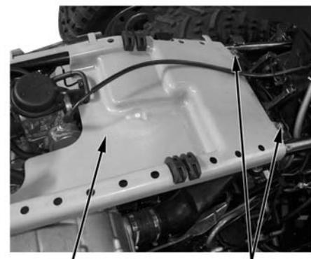
Bottom Plate, Fuel Tank Bolt
