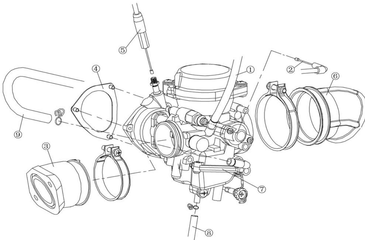
**Note:** Align the installation mark of carburetor and carburetor joint
