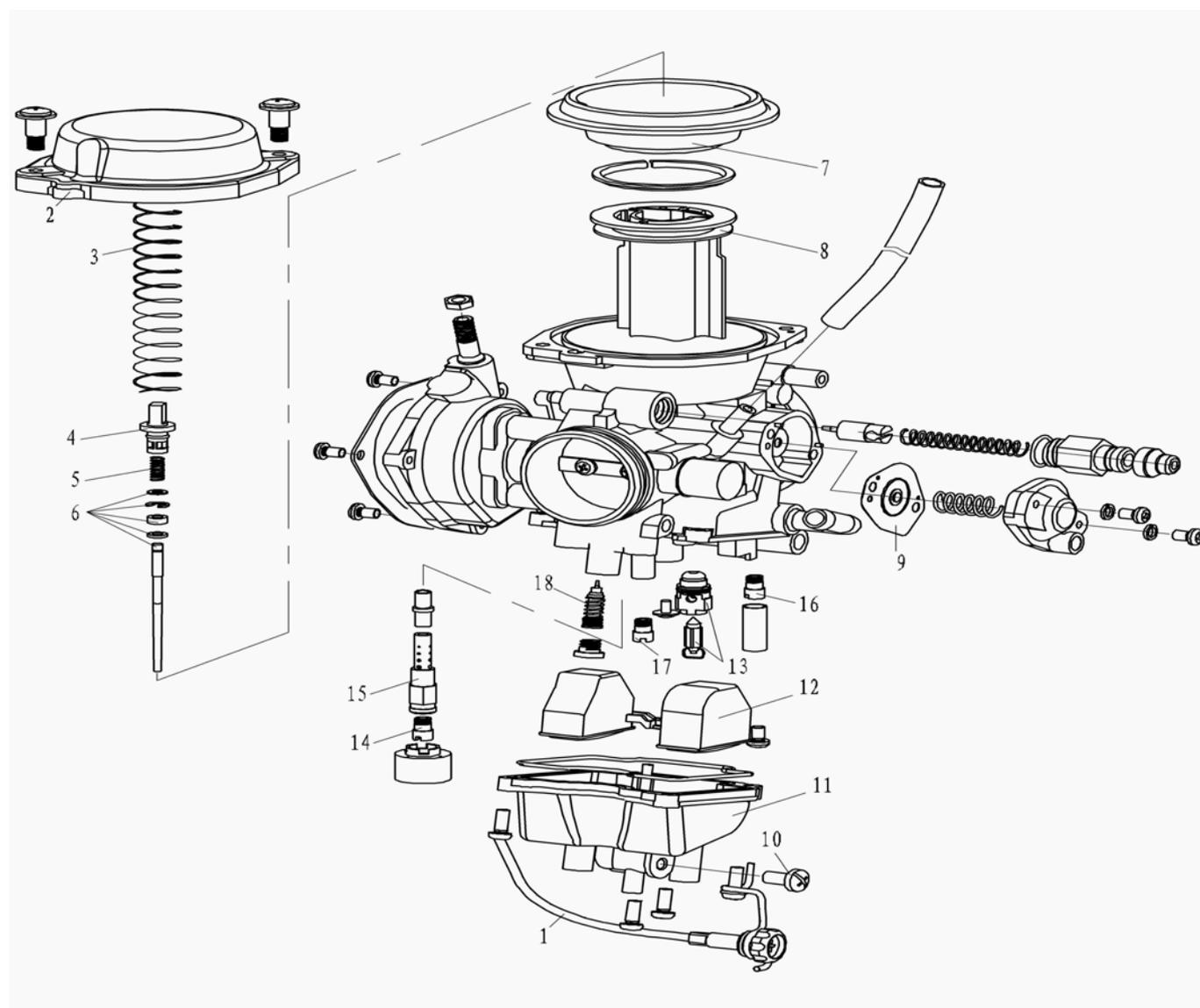
Disassemble the carburetor in the following serial number:
