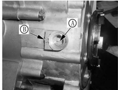
**Note:** while rotating crankshaft, pull the cam chain upward, or the chain will be caught between sprocket and crankcase.
