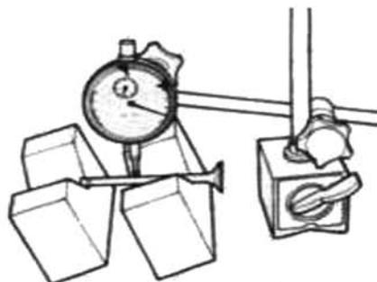
**Valve Head Radial Run-out**
