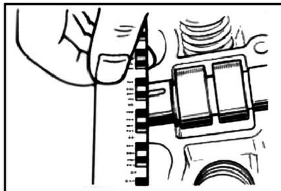
**Note:** Do not turn the camshaft with plastic gauge in place.
