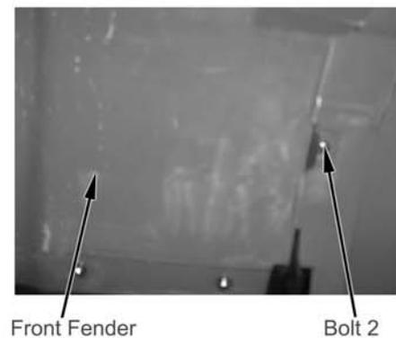
Remove screw for right side panel and right footrest board
