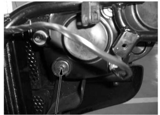
Adjusting Screw, Headlight Beam
