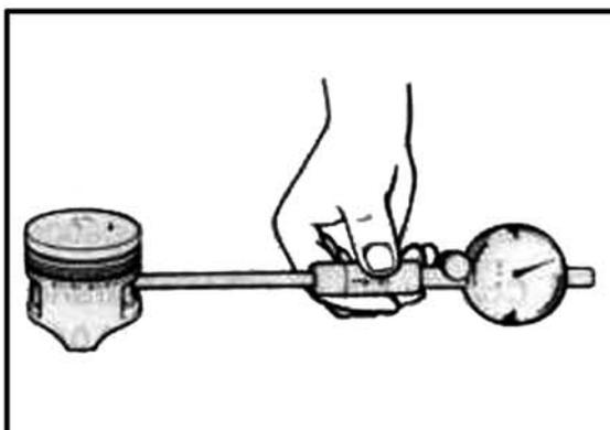
**Piston pin bore limit: 23.030mm**
