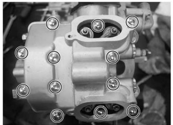
**Gasket Sealant Applying Place**
