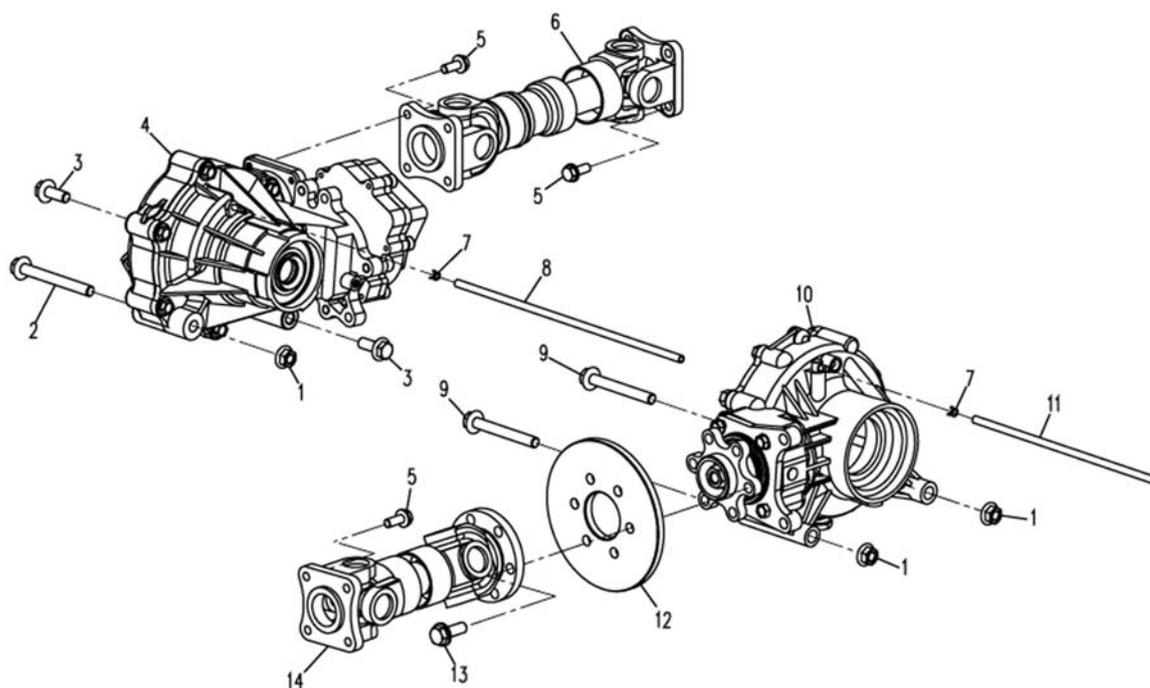
1. Nut    2. Bolt 1    3. Bolt 2    4. Front Axle    5. Bolt 3    6. Front Drive Shaft
