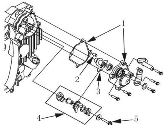
**Driven sector gear tightening torque: 14N.m**
