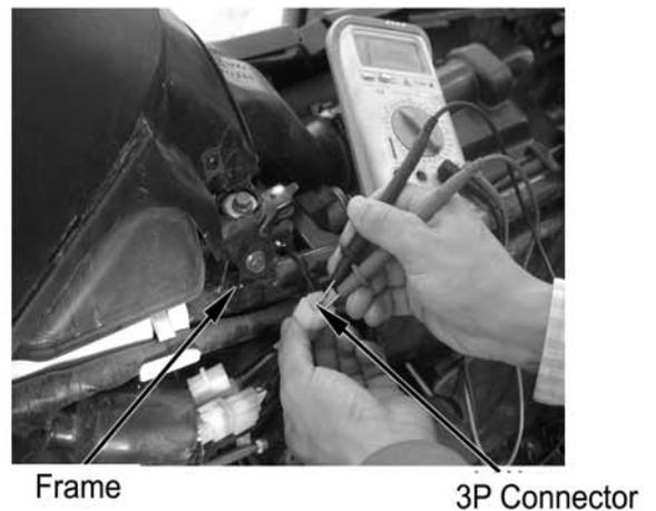
Make sure the yellow terminal of AC magneto 3P connector is not connected with frame body earth wire.
