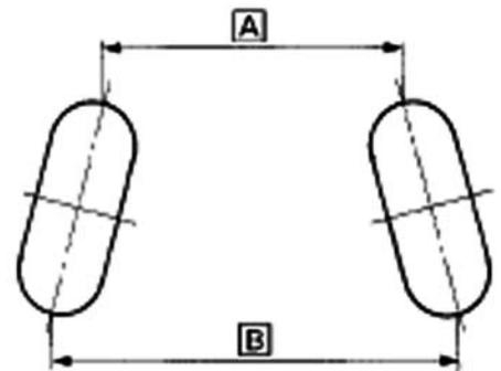
Toe-in out of the range: → Adjust the locknut of tie-rod
