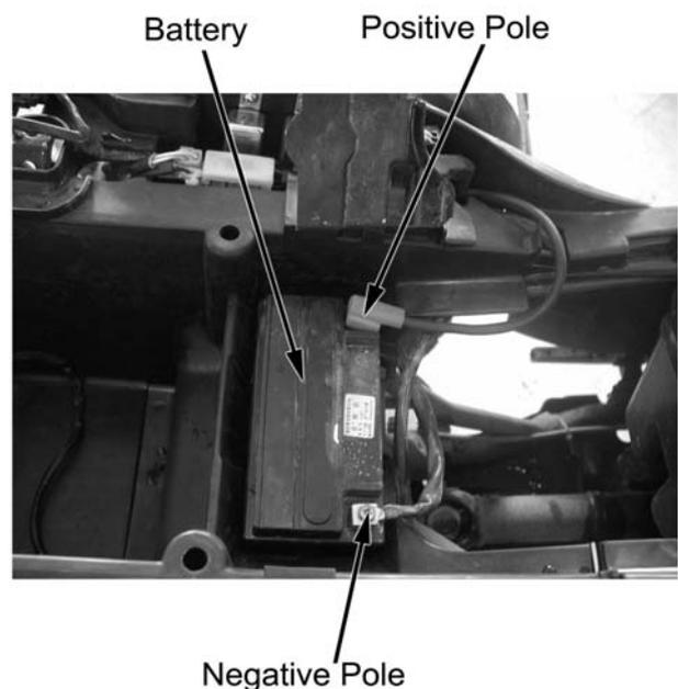
Connect charger's positive wire to battery's positive pole.
