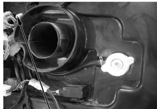
Remove fuel sensor 2P connector.
