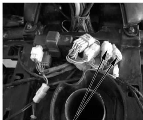
Connector, Handlebar Switch
