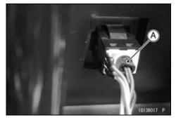
• Pull the bulb [A] out of the socket.
