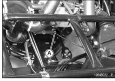
Accessory Fuse 10 A [A] Main Fuse 30 A [B] Battery [C]
