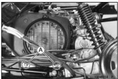
• Remove the stoppers [A] of the fan housing.
