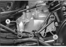
Remove: Driven Bevel Gear Assembly [A]
