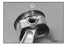
• Remove the piston by pushing the piston pin [A] out the side from which the snap ring was removed.
