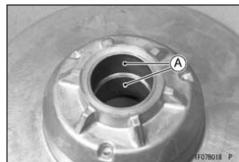
★ If the splines [A] of the fixed sheave [B] and ramp [C] are damaged or worn, replace them.
