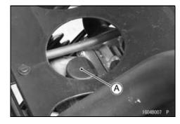
• Apply engine oil to the rubber seal lip [A] on the dipstick.
