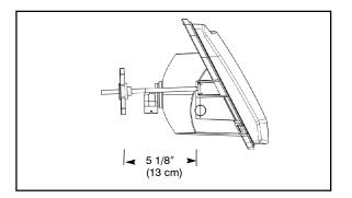
**\*NOTE:** The distance from the headlamp parting line to the end of the adjustment knob stop is 5 1/8, (13 cm). See illustration.
