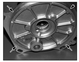
7. Remove large sealing O-Ring from outer edge of stator plate.
