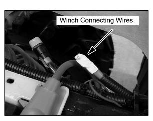
The Orange/White wires are located under the front cover (under headlight pod). The Orange/White wires supply the control power to the winch.
