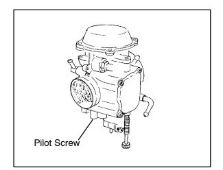
5. Install the pilot mixture screw, spring, washer, and O-ring as an assembly. Lubricate the O-Ring with oil or light grease before installation. CAUTION: Do not damage the O-ring during installation. Turn the screw in until it *lightly* contacts the seat. Back out the specified number of turns. NOTE: The final pilot (idle) mixture must be adjusted with the engine running.
