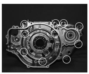
1. Remove flange bolts (10) from magneto side crankcase evenly in a criss-cross pattern.
