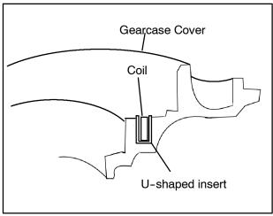
Side Cutaway View of Centralized Hilliard Cover
