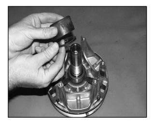
Brass Washer Thickness Standard: .030" (.76mm) Service Limit: .025" (.64mm)
