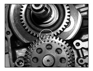
Note the alignment dots on the balancer and crankshaft gears, the marks must be aligned during reassembly.
