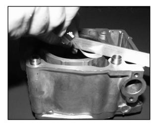
2. Inspect the top of the cylinder for warpage using a straight edge and feeler gauge.
