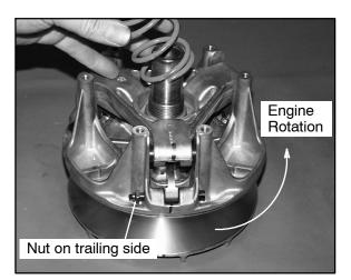
8. Reinstall cover, aligning bosses on the tower and cover. Torque cover bolts evenly to specification
