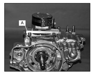
Position the Piston Support Block (PN 2870390) (A) beneath the piston skirt to support the piston during cylinder installation. 3. Apply clean engine oil to the ring compressor (Snap On<sup>™</sup> PN RCL30) and install the compressor following manufacturers instructions. **CAUTION:** Make sure the oil control ring upper rail tab is positioned properly in the notch of the piston. Verify all ring end gaps are correctly located.
