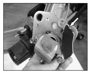
6. Measure the thickness of the pad material. Replace pads if worn beyond the service limit.
