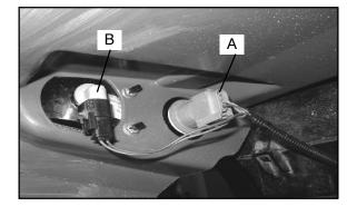
1. To remove the worklight electrical connector (B), pull down on the connector lock and pull the connector from the bulb assembly.
