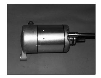
2. Remove the two bolts, washers, and sealing O-Rings. Inspect O-Rings and replace if damaged.
