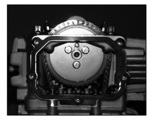
4. Align single (TDC) mark on flywheel with projection in inspection hole, and the cam sprocket pin (facing upward) aligned with the camshaft to crankshaft center line. **NOTE:** The cam lobe should be pointing down and valves should have clearance at this point.
