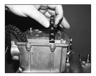
1. Remove cam chain guide at front of cylinder.
