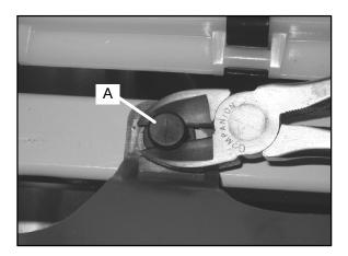
Next, use the diagonal side cutters under outside insert (B) to completely remove the assembly. **NOTE:** The inside insert (A) will still be installed in the outside insert (B
