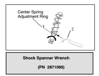
Operator weight and vehicle loading affect suspensionspringpreloadrequirements. Adjustas necessary, using the spanner wrench (2) supplied in your ATV tool kit to turn the adjustment cam (1).
