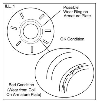
4. Check to make sure the coil is seated in the U-shaped insert that is pressed into the gearcase cover. The top of the coil should be seated below the U-shaped insert. The U-shaped insert controls the pole gap. If the top of the coil is above the surface of the U-shaped insert it raises the armature plate, thereby increasing pole gap. If the pole gap increases the coil will not be strong enough to engage the AWD system. If this is the cause order a new Plate Cover Assembly (PN)
