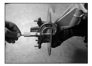
Brake Disc Thickness New .150-.165″ (3.810-4.19 mm) Service Limit .140″ / 3.556 mm
