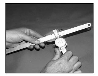
5. Subtract the thickness of the straightedge from the measurement obtained in Step 4 and record.
