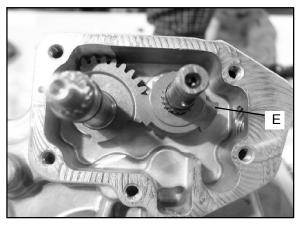
11. Remove the shift shaft (D) and the shift gears.
