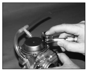
2. Remove float bowl and carefully remove the pressed float pin.
