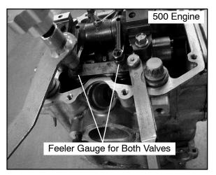
**NOTE:** The exhaust valves share a common rocker arm, and must be adjusted using two feeler gauges.
