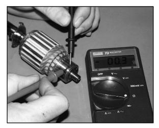
3. Using a digital multitester, measure the resistance between each of the commutator segments. The reading should be .3 ohms or less.
