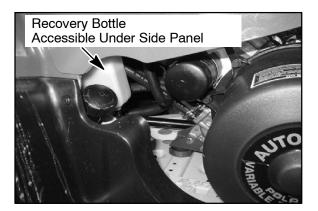
With the engine at operating temperature, the coolant level should be between the upper and lower marks on the coolant reservoir. If not:
