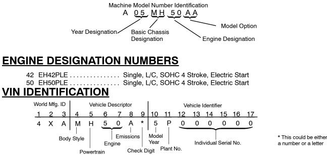
Whenever corresponding about an engine, be sure to refer to the engine model number and serial number. This information can be found on the sticker applied to the recoil housing on the right side of engine.(A) An additional number is stamped on the center top of crankcase beneath the cylinder coolant elbow.
