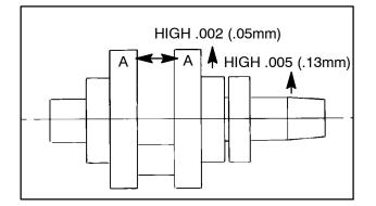
3. If the crank rod pin location is 180° from the dial indicator (opposite that shown above), it will be necessary to spread the crankshaft at position A as shown in the illustration at right. When rebuilding and straightening a crankshaft, runout must be as close to zero as possible.
