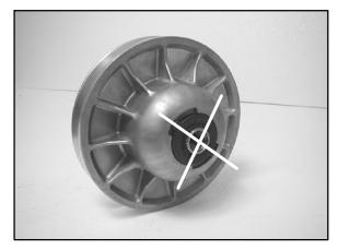
2. It is important to mark the position of the shaft, stop plate, and sheave before disassembly. Mark the helix and inside sheave also. This will aid in reassembly.
