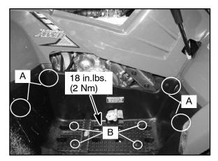
3. Reverse the removal procedures to install the foot well. Be sure to properly align the the cab ends into the foot wells upon reassembly.
