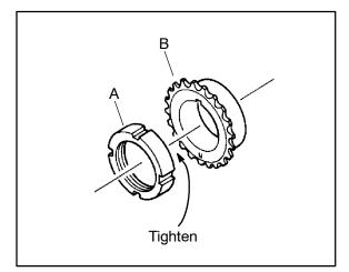
1. Install the Woodruff key, drive sprocket, and slotted nut. Tighten the nut to the specified torque.
