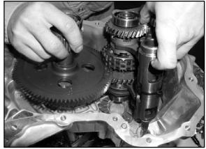
16. With all of the components in the correct positions install the 4 output gear assembly screws. Apply Loctite <sup>™</sup> 262 (PN 2871952) to the threads of the screws. Torque the screws to 8–12 ft.lbs. (11–16 Nm). NOTE: If the transmission is in locked in Park take it out of gear.
