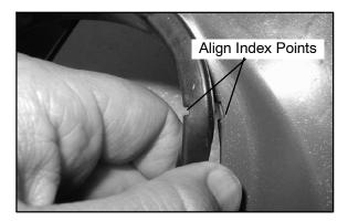
3. Hold the pod assembly securely and insert the instrument cluster into the pod assembly. Twist the instrument cluster gently in a clockwise motion to properly seat the instrument cluster into the pod assembly. Apply pressure on the bezel while pressing down on the instrument cluster.
