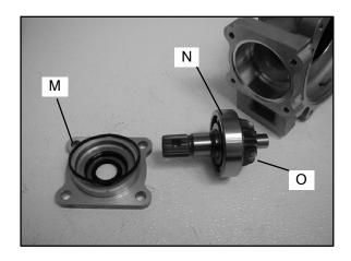
17. Inspect the output shaft bushing. Replace as needed. Clean the inside surfaces of both gearcase halves.
