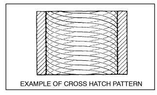
A finished cylinder should have a cross-hatch pattern to ensure piston ring seating and to aid in the retention of the fuel/oil mixture during initial break in. Hone cylinder according to hone manufacturer's instructions, or these guidelines:
