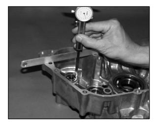
2. Measure the distance from the magneto crankcase mating surface to the bearing using a dial caliper and a straight edge. Subtract the thickness of the straightedge and record.
