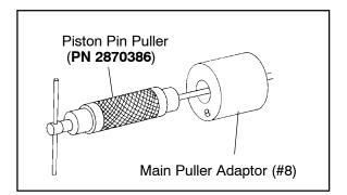
3. Install the Main Puller Adapter (#8) (**PN 5020632**) onto the Piston Pin Puller (**PN 2870386**).
