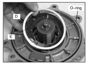
Inspect the armature plate (E) for a consistent wear pattern. Uneven wear of the armature plate (E) indicates a warped plate, which may cause intermittent operation. **NOTE:** See "FRONT GEARCASE DIAGNOSIS" later in this chapter for more details.
