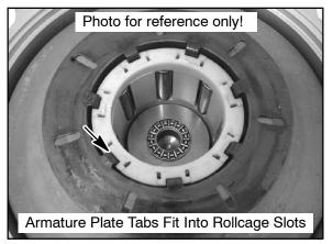
**NOTE:** This photo is for reference only, the armature plate is actually installed in the output cover.
