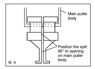
4. Ensure that the split between the puller legs is fully supported by the main body of the tool (III 4).
