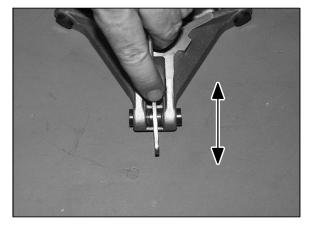
4. Rubber backed buttons can and should be used in all ATV clutches *if the hollow roller pin is changed to a solid roller pin.* **NOTE:** The rubber side of the
