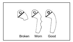
Inspect the weight pivot bore and pivot bolts for wear or galling. If weights or bolts are worn or broken, replace in sets of three with new bolts. **NOTE:** A damaged shift weight is usually caused by a damaged or stuck roller in the spider assembly. See roller inspection, Page 6.12.
