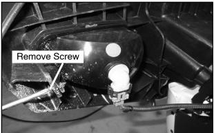
3. To remove the headlamp, firmly press on front of headlight and replace with a new headlamp.
