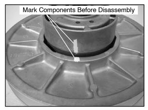
Place the driven assembly into the clutch holder. Push helix inward. Remove snap ring (A) and washer (B). NOTE: The spring is a compression
