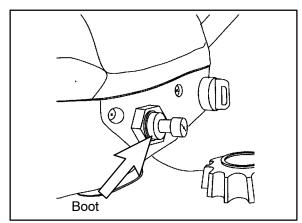
If the choke knob does not stay out when pulled, adjust the choke tension by tightening (clockwise) the jam nut under the rubber boot between the choke knob and nut. Firmly grasp the rubber boot and tighten until the choke slides freely but stays out when pulled.
