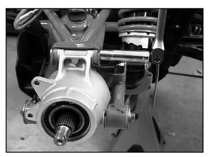
Install hub, flat washer, domed washer (domed side out) and nut. Torque center hub nut to 80 ft. lbs. (109 Nm). Install new cotter pin and hub cap.
