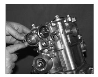
4. Remove camshaft end cap and O-Ring.
