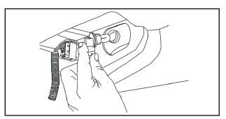
**\*NOTE:** Do not touch the lamp with bare fingers. Hold the plastic part (1) of the lamp. Oil from your skin leaves a residue, causing a hot spot that will shorten
