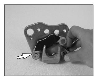
3. Remove mounting bracket, pin assembly and dust boot.
