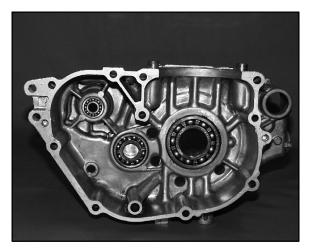
1. Make sure all bearings are firmly seated in the both Mag and PTO crankcase.
