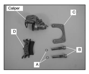
5. Remove the anvil bolts and separate caliper halves and remove pistons with piston pliers.
