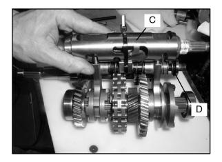
15. With the gearcase on it's side, hold the gear cluster assembly and output assembly together. Carefully install each shaft into their respective recess in the gearcase.
