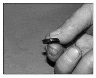
13. Remove ratchet pawl with spring and inspect. Replace spring or ratchet pawl if worn, broken, or damaged.
