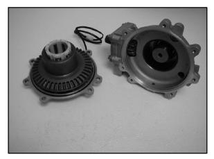
**NOTE:** Be careful not to misplace the thrust bearing located between the two output shafts.
