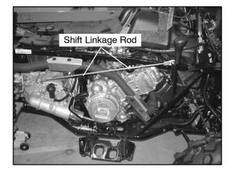
Inspect shift linkage tie rod ends, clevis pins, and pivot bushings and replace if worn or damaged. Lubricate the tie rod ends with a light aerosol lubricant or grease. 2. Note orientation of tie rod end studs with the ends that are up down (vertical). Remove both rod end bolts from transmission bell crank.
