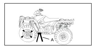
4. Remove the wheel nuts and remove the wheel.
