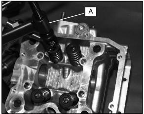
Using a valve spring compressor (A), compress the valve spring and remove the split keeper.
