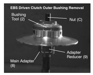
10. Remove bushing and removal tool from adapters. Discard bushing.
