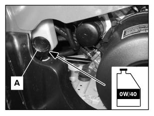
The oil tank is located on the left side of the vehicle. To check the oil level:
