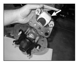
4. Push caliper piston into caliper bore slowly using a C-clamp or locking pliers with pads installed.
