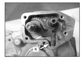
27. Install the park lockout assembly. Torque the park lockout to 14–18 ft.lbs. (19–24 Nm).
