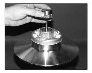
Install sheave onto puller with new bushing upward as shown. Install the Number Two Puller Adapter (#10) (PN 5020633).
