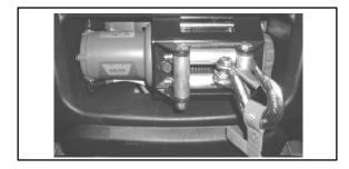
The mini-rocker (IN/OUT) control controls the direction of the cable for the winch. IN pulls the cable into the winch and OUT feeds the cable out of the winch.
