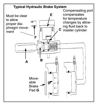
The Polaris disc brake system consists of the following components or assemblies: brake lever; master cylinder; hydraulic hose; brake calipers (slave cylinder); brake pads; and brake discs, which are secured to the drive line.
