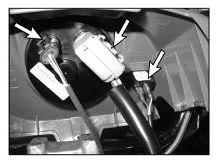
2. Push the instrument cluster out from the backside of the pod, while securely holding the pod.
