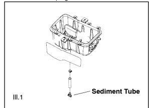
**NOTE:** The sediment tube will require more frequent service if the vehicle is operated in wet conditions or at high throttle openings for extended periods.
