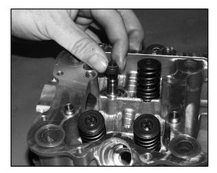
5. Remove valve seals. **CAUTION:** Replace seals whenever the cylinder head is disassembled. Hardened, cracked or worn valve seals will cause excessive oil consumption and carbon buildup.
