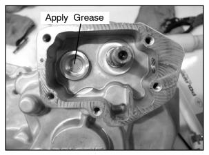
23. Install the shift gear (16T) (G) on the shift drum shaft. Install the sector gear (F) in the bushing pocket on the left side. Aligning the timing marks on the gears.
