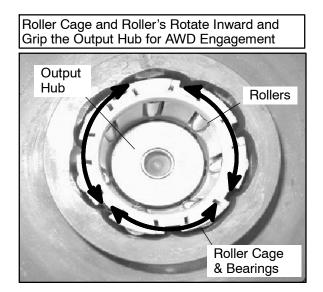
**Disengagement:** As the front and rear wheels gain traction, rotating very close to the same speed, the front wheels "overdrive" the output hubs and the rollers are forced outward, disengaging the AWD. The vehicle is now back to rear wheel drive until the next loss of traction.
