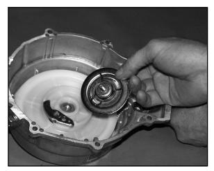
12. Inspect plate for wear or damage. Inspect plate friction spring for wear, damage, and proper tension. The spring should fit tightly on friction plate.
