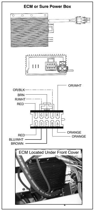
The ECM (Sure Power Box) integrates three electronic features found on the Polaris ATV. These features are alternator rectifier/regulator, engine temperature controller, and solid state circuit breaker outputs.
