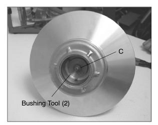
3. Using a hand held propane torch, apply heat around outside of bushing until tiny smoke tailings appear.
