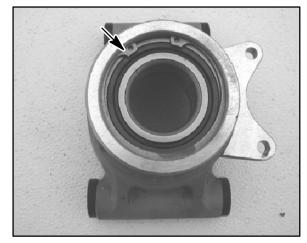
2. From the back side, tap on the outer bearing race with a drift punch in the reliefs as shown.
