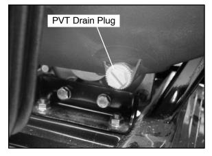
To drain any water that may be trapped inside the PVT cover, simply remove the PVT drain plug and O-ring located on the bottom of the PVT cover and let the water drain out. The PVT drain plug is shown below.
