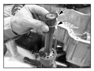
34. To remove the snorkel shaft from the snorkel tube, use a press to press the snorkel shaft out.
