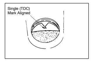
Disconnect the wire from the cam chain and rotate the engine to align the <u>single</u> (TDC) timing mark (Top Dead Center) on the flywheel with the notch in the timing inspection window. Be sure to use the *single* TDC mark when installing the cam. Do not use the advance marks. See III. on next page.
