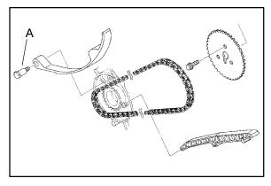
1. Remove bolt securing tensioner blade to crankcase (A).
