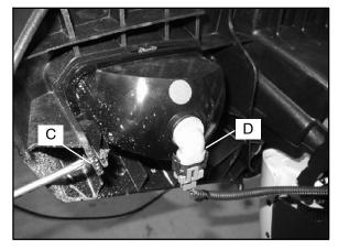
8. Remove the remaining bolts and screws that secure the front bumper section to the frame.
