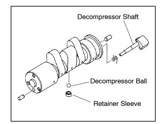
10. Slide camshaft out the PTO side of the cylinder head.
