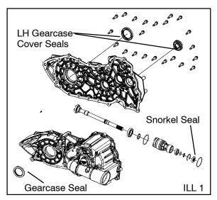
2. Reverse the disassembly procedure for the assembly of the snorkel shaft assembly.
