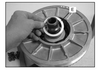
5. Inspect surface of rollers for flat spots and wear. Rollers must rotate freely on pins without excessive clearance. Check the roller pin and roller bore for wear and replace if necessary.
