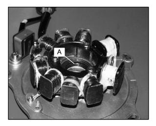
5. Replace crankshaft seal (A).
