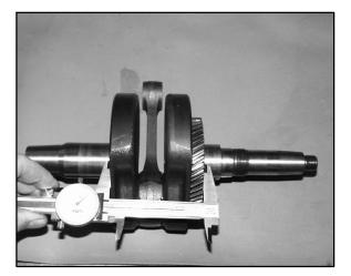
7. Measure the width of the crankshaft at the bearing seats with a micrometer or dial caliper and record.
