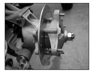
Rear Hub Nut Torque: 80 ft. Ibs. (109 Nm)
