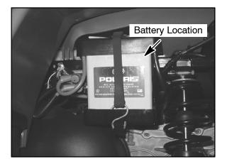
Inspect the battery fluid level. When the battery fluid nears the lower level, remove the battery and fill with <u>distilled water only</u> to the upper level line. To remove the battery:
