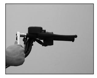
2. Place a shop towel under brake line connection at master cylinder. Loosen banjo bolt; remove bolt and sealing washers.
