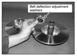
7. Remove moveable sheave and note the number of spacer washers. One spacer must remain between the sheaves when adjusting belt deflection.
