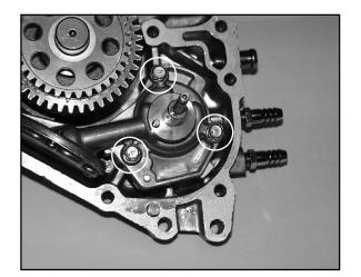
4. Remove three oil pump retaining bolts and pump.
