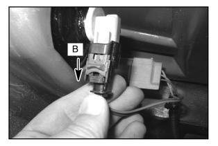
2. To remove the brake light electrical connector (B), press in on the tab on the connector to unlock the connector and pull the connector from the bulb assembly.
