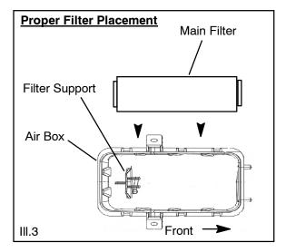
**NOTE:** The air filter should rest on the filter support. Proper placement of the air filter is important to prevent rattles and air leaks. See Illustration above.
