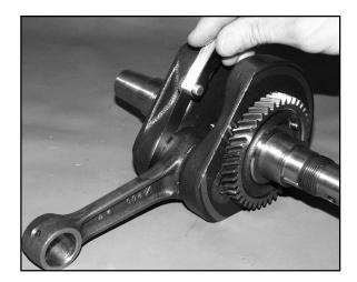
3. Use a feeler gauge to measure the connecting rod big end side clearance.
