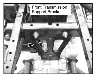
17. Remove bottom transmission bolts as shown in Illustration below. The bolts are accessible through the skid plate.
