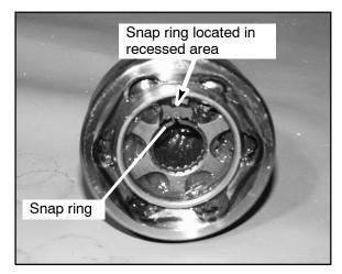
3. Open the snap ring using a snap ring pliers or small needle nose pliers. Tap CV housing off shaft with a soft faced hammer while holding snap ring open.
