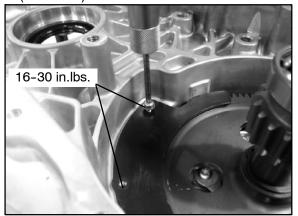
18. Install the 59T rear drive sprocket and drive chain.
