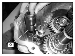
19. Remove the output gear (M) and gear cluster assembly from the gearcase by pulling both assemblies straight up. Place the gear cluster assembly on a clean surface for inspection.
