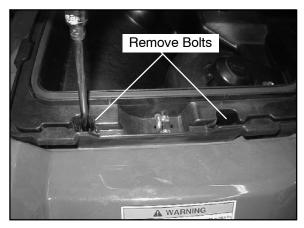
5. Remove the two (T25) screws that secure the outside of the storage box to the front fenders (each side).
