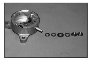
8. Remove the electrical tape and reinstall the two small phenolic washers, the large phenolic washer, flat washer, and nut.
