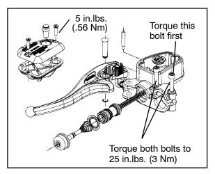
**NOTE:** To speed up the brake bleeding procedure, the master cylinder can be purged of air before brake line is attached. Fill with DOT3 Brake Fluid (**PN 2870990**) and pump lever slowly two to three times with finger over the outlet end to purge master cylinder of air.
