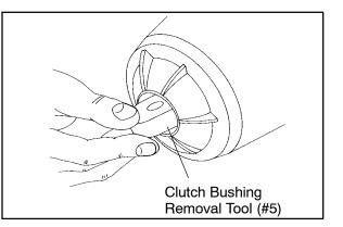
Working from the top, install Driven Clutch Bushing Removal Tool (#5) (PN 5020631) into the center of clutch sheave with smaller diameter toward bushing to be removed. See illustration.
