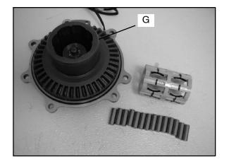
10. Install the rollers and roll cage into the ring gear. Insert the rollers as the roll cage is installed.
