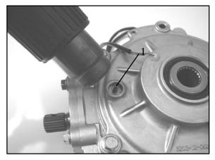
Using a hex wrench, turn the back-lash screw out 3-4 turns. Re-apply red loctite onto the bottom screw threads.
