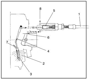
Fuel is drawn into the starter circuit from the float chamber (2) through the starter jet (3). Starter jet meters this fuel, which then flows into starter pipe (4) and mixes with the air (7) coming from the float chamber. The mixture, rich in fuel content, reaches starter plunger and mixes again with the air coming through a passage (8) extending from underneath the diaphragm. The rich fuel/air mixture for starting is discharged through starter outlet (6) in the the main bore.
