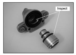
11. Inspect surface of caliper piston for nicks, scratches, or damage and replace if necessary.
