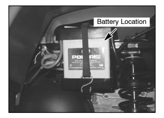
NOTE: All 2005 Sportsman 400/500 ATV batteries are Low Maintenance in design and construction. All Low Maintenance batteries are fully charged and tested at the factory before installation. Expected shelf life is 6-8 months depending on storage conditions. As a general rule before placing the battery into service, check the battery condition and charge accordingly.
