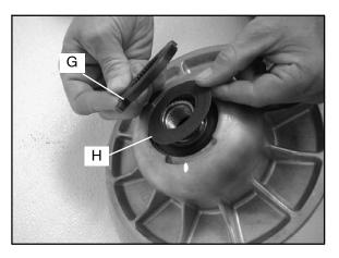
11. Remove the shaft (I) from the sheave assembly. Inspect washers and bearing for wear.
