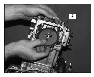
4. Loop the cam chain on the cam sprocket with the dots on the sprocket facing outward and the alignment pin notch facing directly upward.
