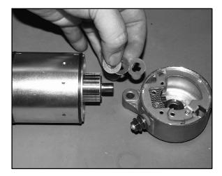
4. Remove shims from armature shaft. **NOTE:** All shims must be replaced during reassembly.
