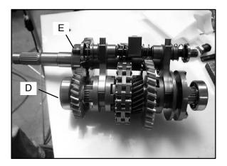
**NOTE:** To ease assembly use a plastic tie strap to hold the shift forks (D) and the shift drum (C) together during assembly.
