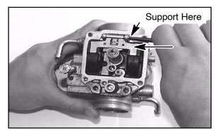
**NOTE:** Be careful not to damage the float pin tower during the float pin removal. Support the float pin tower while removing the float pin. This helps to prevent the float pin towers from breaking off.
