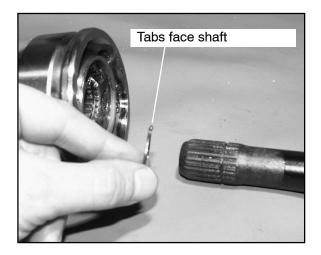
5. Refit CV joint on interconnecting shaft by tapping with a plastic hammer on the joint housing. Take care not to damage threads on the outboard CV joint. The joint is fully assembled when the snap ring is located in the groove on the interconnecting shaft.
