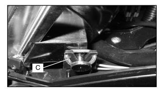
5. Pull the headlight housing up to release from the locking tabs.
