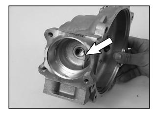
18. Remove and replace the O-rings and seals from the assembly.
