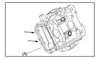
Thoroughly clean cylinder head (A) surface to remove all traces of gasket material and carbon.
