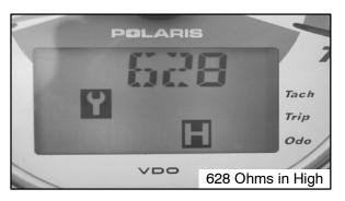
**Screen 5: Programmable service interval.** The purpose of the programmable service interval is to provide the consumer and dealer with a convenient reminder for routine maintenance. When the ATV leaves the factory, this feature is set at 50 hours.
