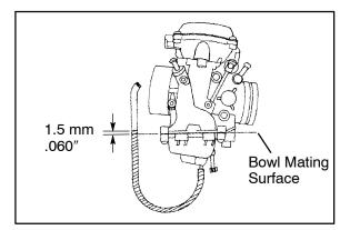
Open bowl drain screw by turning counterclockwise approximately two turns. Start and run engine for 3 to 5 seconds to allow fuel level to stabilize in the line. If level is out of specification, remove carburetor and inspect inlet needle and seat, float height, passages, etc.
