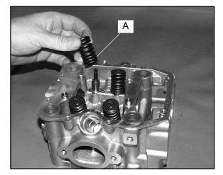
2. Remove spring retainer and spring.
