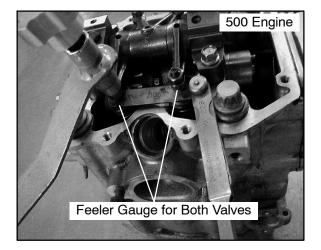
**NOTE:** The exhaust valves share a common rocker arm, and must be adjusted using two feeler gauges.
