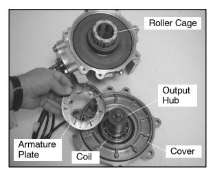
**4x4 Engagement:** When the AWD switch is activated, a 12 VDC current charges the central coil which creates a magnetic field. This magnetic field attracts an armature plate keyed to a roller cage that contains 14 rollers and roller cam. The difference in rpm by input shaft and front axles the forces the rollers up the external cam. The rollers engage themselves to the output hubs that link both front axles, resulting
