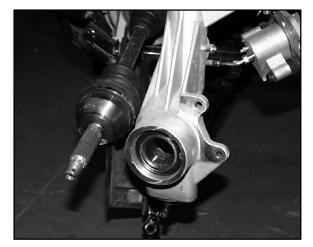
11. With short, sharp jerks, remove drive shaft from front gearcase.
