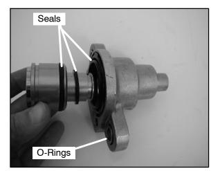
2. Carefully assemble caliper body, making sure O-rings are properly positioned in groove. Tighten the caliper anvil bolts and then torque the anvil bolts evenly to 16-18 ft. lbs. (22-25 Nm).
