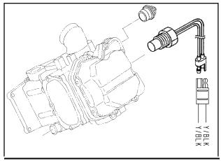
If the thermistor circuit is open the engine Hot light and fan will both come on. With engine cold, disconnect lead and measure resistance of sensor between the two Yellow/Black connector terminals. There should be no continuity or very high resistance (see chart below).
