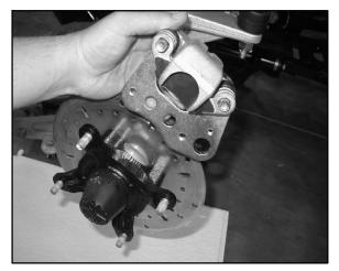
**CAUTION:** Do not hang the caliper by the brake line. Use wire to hang the caliper to prevent possible damage to the brake line.
