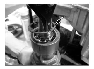
33. Remove the second snap ring and spacer from the snorkel shaft.
