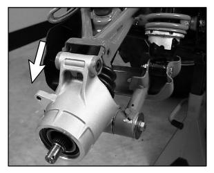
3. Pull sharply outward to remove shaft from transmission. Install a new lock ring upon assembly.
