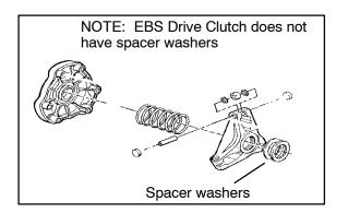
6. Reinstall shift weights using new lock nuts on the bolts.
