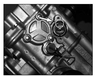
Install the thermostat with one of the air bleed holes positioned next to the upper thermostat cover bolt hole as shown.
