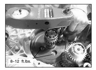
17. Install the oil deflector shield into the gearcase. Apply Loctite <sup>™</sup> 262 (**PN 2871952**) to the threads of the screws. Torque the screws to 16–30 in.lbs. (2–3.3 Nm).
