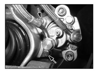
5. Push caliper pistons into caliper bore slowly with pads installed.
