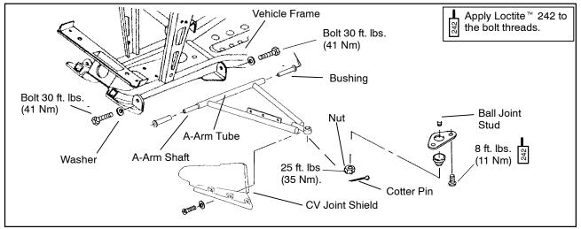
8. Install new A-arm assembly onto vehicle frame. Torque new bolts to 30 ft. lbs. (41.4 Nm).
