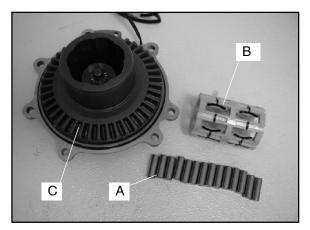
8. Inspect roll cage (B) sliding surface. This surface must be clean and free of nicks, burrs or scratches. Remove and inspect the H-springs.
