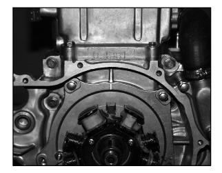
4. Install the stator plate being careful not to damage the seal. Align timing reference marks on the plate and crankcase. Be sure the plate is fully seated.
