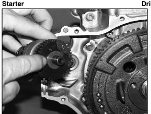
1. Be sure the washer is positioned on the back of the drive gear.
