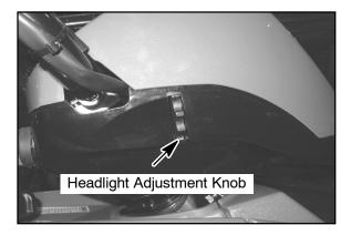
1. Place the vehicle on a level surface with the headlight approximately 25' (7.6 m) from a wall.
