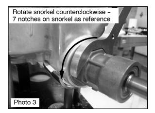
8. Once the gear backlash is found, to install the snorkel lock screw, you may have to rotate the snorkel tube clockwise or counterclockwise slightly. This will allow the snorkel lock screw to thread itself into one of the slots of the snorkel tube (See illustration below) to secure the snorkel tube.
