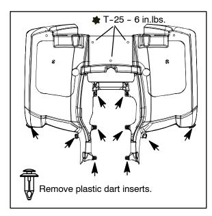
4. Disconnect the rear lights by pulling the locks on each side and removing the connectors. Lift the rear cab from the frame.
