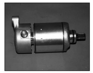
3. Remove brush terminal end of housing while holding other two sections together.
