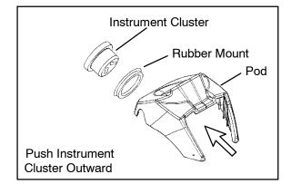
**\*NOTE:** Do not remove the rubber grommet in the pod. Only remove the rubber grommet if necessary.
