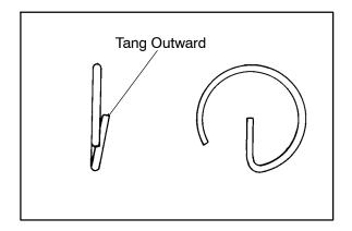
3. Install a new circlip on one side of the piston with the end gap facing *up* or *down*, and tang outward.
