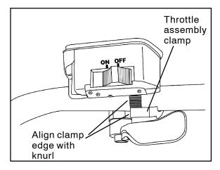
Align throttle control assembly clamp with knurl on handlebar
