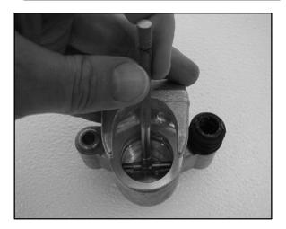
2. Inspect piston for nicks, scratches, wear or damage. Measure diameter and replace if damaged or worn beyond service limit.
