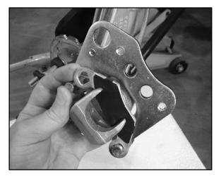
3. Install caliper on hub strut, and torque mounting bolts.
