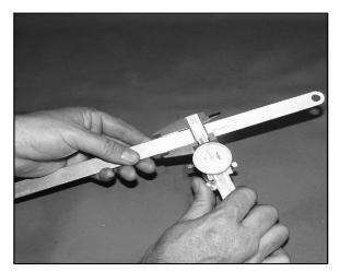
3. Subtract the thickness of the straightedge from the measurement obtained in Step 2 and record.
