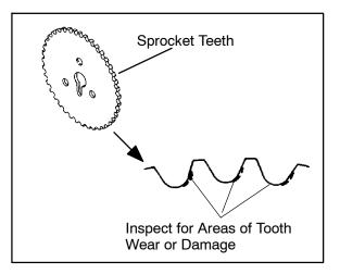
9. Inspect cam sprocket teeth for wear or damage. Replace if necessary.
