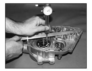
2. Measure the distance from the PTO crankcase mating surface to the main bearing using a dial caliper and a straight edge.
