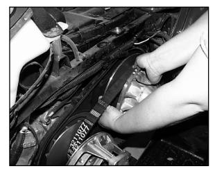
3. The belt then should be able to be pushed down into and between the sheaves.
