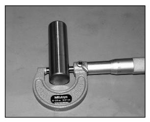
3. Measure O.D. of rocker shaft. Inspect it for wear or damage. Compare to specifications.
