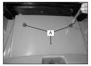
3. Remove the ten plastic inserts that secure the rear cab to the frame and plastic.
