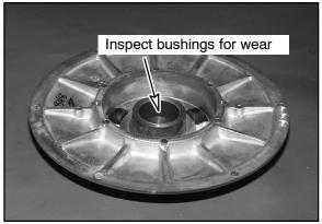
Moveable Sheave Bushing Inspection: Replace the bushing if more brass than Teflon<sup>™</sup> is visible on the bushing. Refer to bushing replacement in this chapter.
