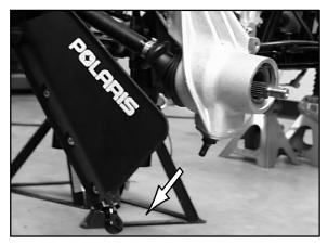
8. Pull the hub and strut assembly out and pull the drive-shaft out of the hub.
