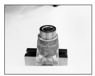
3. Press bearing into place until outer race bottoms on housing.
