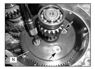
18. Remove the shift drum (O) from the gearcase by moving the drum up and to the right to clear the shift shaft.
