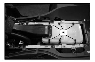
4. Loosen clamp and remove air filter assembly.
