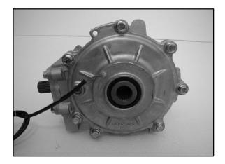
Front Gearcase Coil Resistance: 22.8-25.2 Ohms
