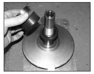
Inspect surface of shaft for pitting, grooves, or damage. Measure the outside diameter and compare to specifications. Replace the drive clutch assembly if shaft is worn or damaged.
