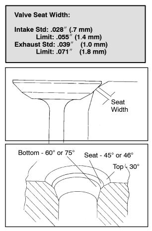
**NOTE:** When using an interference angle, the seat contact point on the valve will be very narrow, and is a normal condition. Look for an even and continuous contact point on the black marker, all the way around the valve face.
