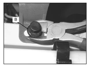
3. To install the inserts, press outside insert (B) into the hole. Press inside insert (A) until it snaps into place.
