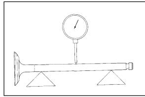
Check valve face for runout, pitting, and burnt spots. To check for bent valve stems, mount valve in a drill or use "V" blocks and a dial
