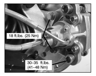
Caliper Mounting Bolt Torque: 18 ft. lbs. (24 Nm)
