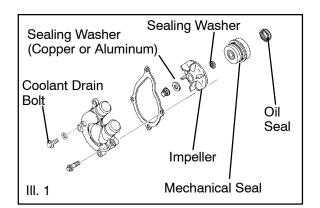
1. After the coolant has been drained, remove the water pump cover, impeller and the sealing washer. (III. 1)
