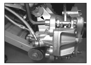
4. Remove caliper mounting bolts and lift caliper off of disc.
