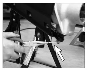
3. Disconnect A-arm from ball joint using a tie rod fork.
