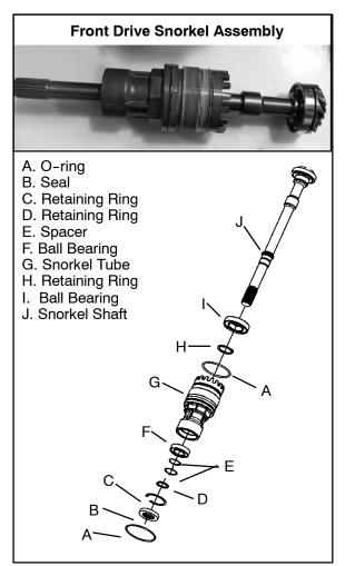
32. If needed, remove the seal from the front of the snorkel tube. Remove the snap ring.
