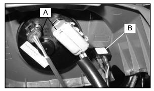
4. Turn the headlight lamp socket counter-clockwise and remove.
