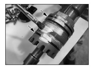
Install the snorkel shaft assembly into the gearcase. Install the snorkel shaft assembly in until the second O-ring is contacting the gearcase, but is still visible.
