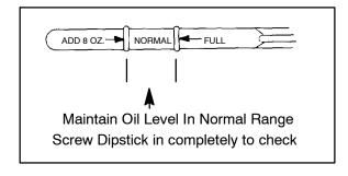
5. Remove dipstick and check to see that the oil level is in the normal range. The oil should be between the top line and the bottom line on the dipstick. Add oil as indicated by the level on the dipstick. Do not overfill.
