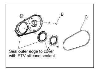
Inner Cover Bolt Torque (Rear): 12 ft. lbs. (16.6 Nm)
