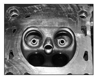
Clean all accumulated carbon deposits from combustion chamber and valve seat area with a soft wire brush.
