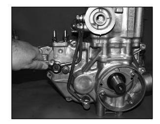
2. Loosen all four oil pipe banjo bolts and then remove the bolts and eight sealing washers. Remove the pipes.
