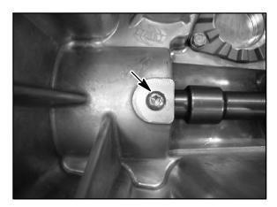
30. Mark the snorkel tube and case with a white pen or marker. This is used to ease reassembly of the gearcase.
