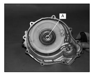
10. Pull recoil rope so it is extended approximately 12-18". Check handle c-ring for proper tension, and the handle for cracks or damage which may allow water or dirt to enter the recoil housing through the rope. **NOTE:** The handle must seal tightly on the recoil housing to prevent water from entering. 11. Remove center bolt from recoil friction plate (A).
