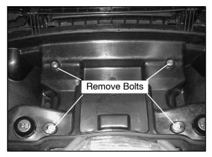
4. Remove the two (T25) screws that secure the storage box to the front fender well areas (each side).
