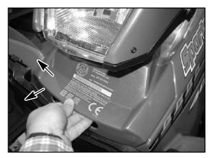
3. To install the front cover, insert the tabs of the front cover into the inserts of the cab. Make sure the tabs are aligned with the slots. Then press the rear tabs into the slots.
