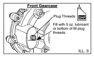
5. Install fill plug and check for leaks.
