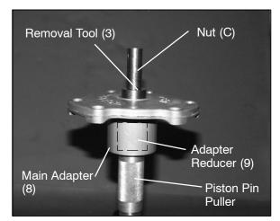
**EBS Drive Clutch Cover Bushing Removal**
