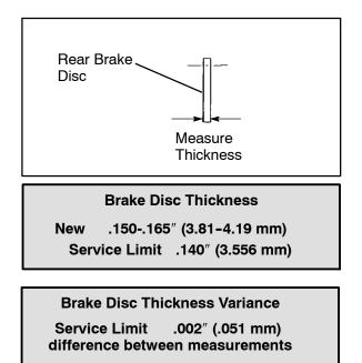
3. Mount dial indicator and measure disc runout. Replace the disc if runout exceeds specifications.
