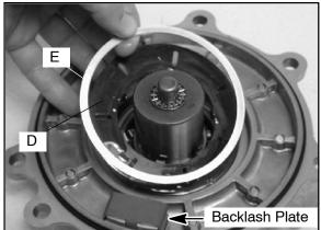
8. Install the retaining ring (F) into the output cover. Be sure the retaining ring is properly seated into the cover.
