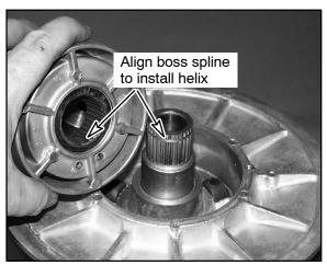
4. Line up boss spline and push helix down until it engages the splines 1/2" to 3/4".
