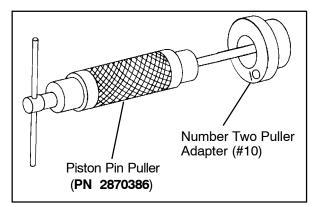
1. Working from the top, insert Number Two Puller Adapter (#10) (**PN 5020633**) onto the puller. See illustration at above.  Start new bushing evenly in moveable sheave. Apply Loctite<sup>™</sup> 680 (PN 2870584) to the back side of new bushing.
