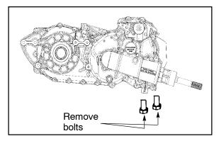
18. Lift and remove transmission out right side of frame.
