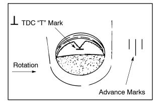
To position crankshaft at Top Dead Center (TDC) on compression stroke:
