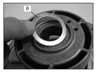
**NOTE:** Rotating the moveable sheave so that the rollers are not in contact with either helix ramp surfaces will lessen the effort needed to push the helix inward.
