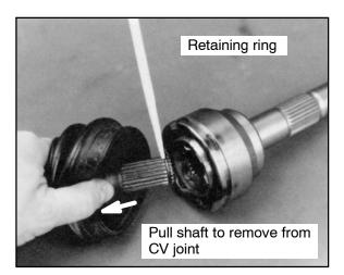
7. Remove small clamp and boot from driveshaft.
