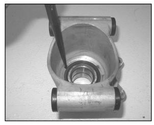
**NOTE:** Drive bearing out evenly by tapping on outer race only. Once bearing is at bottom of casting, support casting on outer edges so bearing can be removed.
