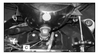
4. Remove O-Ring (C) from headlight pivot pins. (Both Sides)
