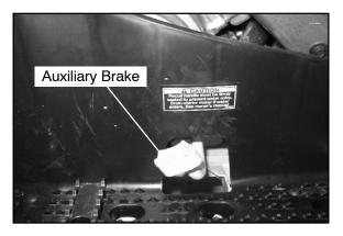
Use the following procedure to inspect the hydraulic auxiliary (foot) brake system and adjust or bleed if necessary:
