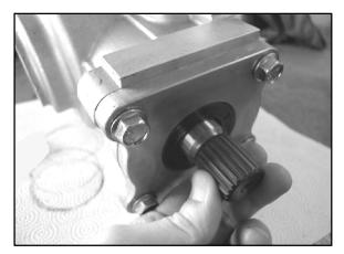
19. If a tight spot is felt during rotation, loosen the backlash screw another 1/8 turn. Perform the previous step again. Repeat this procedure until the pinion shaft rotates smoothly 4 times (1 revolution of ring gear).
