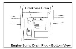
18. Approximately 1 cup of engine oil will remain in the crankcase. To drain, remove drain plug found on lower right side of crankcase.
