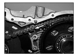
Remove the cam chain tensioner spring (J). Slide the cam chain tensioner shoe (G), pins (H), and cam chain tensioner cam (I) from the assembly.
