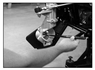
**NOTE:** Drive bearing out evenly by tapping on outer race only. Once bearing is at bottom of casting, support casting on outer edges so bearing can be removed.
