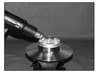
4. Using a hand held propane torch, apply heat directly on bushing until tiny smoke tailings appear.
