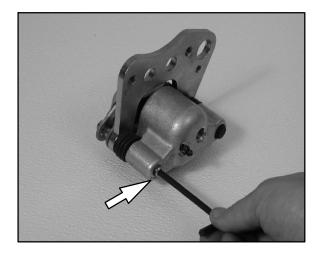
2. Push upper pad retainer pin inward and slip brake pads past edge.
