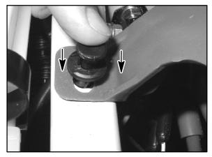
The inside insert (A) should be flush with the top of the outside insert (B).
