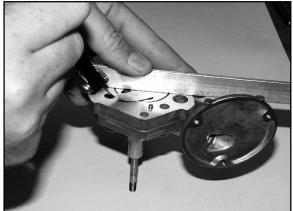
9. Measure pump end clearance using a feeler gauge and straight edge.
