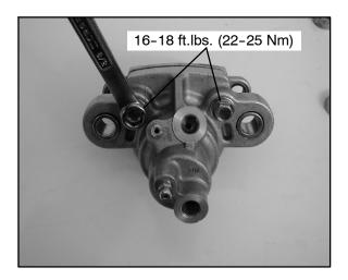
**Caliper Anvil Bolt Torque:** 16-18 ft. lbs. (22-25 Nm)
