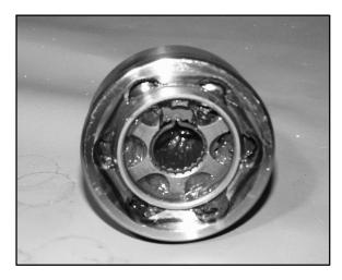
4. Add the recommended amount of grease for *CV joint cleaning* to the joint as shown below. Be sure grease penetrates all parts of the joint.
