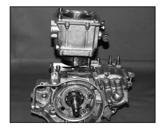
4. Apply clean engine oil liberally to the cylinder bore and tapered area of the sleeve. Install the cylinder with a slight rocking motion until the rings are captive in the sleeve.
