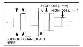
1. To correct a situation like the one shown in the illustration at right, strike the shaft at point A with a brass hammer.
