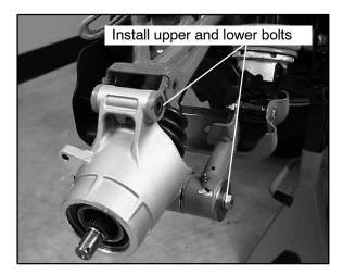
Lower Control Arm Bolt Torque: 40 ft. lbs. (54 Nm)
