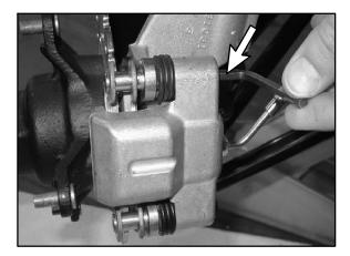
3. Remove caliper from mounting bracket.
