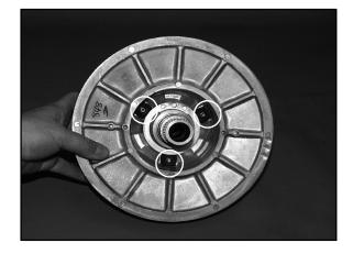
Inspect ramp buttons in the moveable sheave and replace if worn. NOTE: The ramp buttons are secured by Torx<sup>™</sup> screws (T20).
