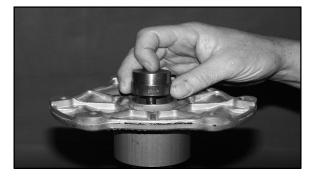
1. Apply Loctite<sup>™</sup> 680 (**PN 2870584**) to the back side of new bushing. Working from inside of cover, insert bushing and bushing installation tool into center of clutch cover.
