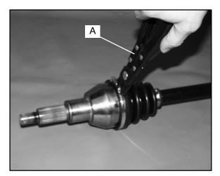
2. **NOTE:** Photo below is shown without shaft for clarity. Wipe grease away from recess in CV joint inner hub to locate snap ring.
