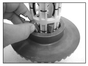
11. Install the output cover assembly onto the main gearcase.
