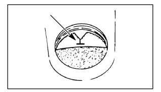
7. Verify accurate TDC positioning by observing the "T" mark aligned with the pointer in the timing inspection hole. In this position there should be clearance on all valves.
