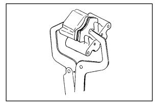
**NOTE:** Brake fluid will be forced through compensating port into master cylinder fluid reservoir when piston is pushed back into caliper. Remove excess fluid from reservoir as required.
