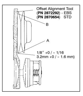
2. With tool touching rear of driven clutch inner sheave, the distance at point "A" should be 1/8".
