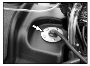
7. Slowly lift the sender out of the tank. Lift the sender out at an angle, so the float will more easily come out of the fuel tank.
