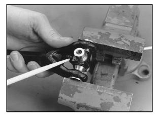
Install new bearing caps in yoke by hand. Carefully install U-joint cross with grease fitting properly positioned inward toward center of shaft. Take care not to dislodge needle bearings upon installation of cross joint. Tighten vise to force bearing caps in.
