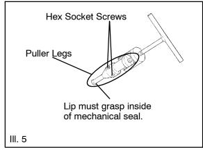
5. Tighten the hex socket screws on the puller legs sufficiently so the lip of the puller legs will grasp the mechanical seal. Ill. 5
