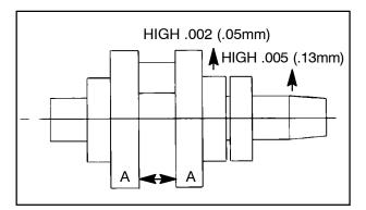
2. To correct a situation like the one shown in the illustration at right, squeeze the crankshaft at point A. (Use tool from alignment kit).
