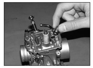
4. Remove the pilot mixture screw, spring, flat washer, and O-Ring. If an anti-tamper plug is installed over the pilot screw cavity, it must be removed for access.
