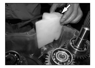
Apply a continuous bead of Crankcase Sealant (3-Bond) (PN 2871557) to the LH gearcase mating surface and install the cover. Install and tighten the 22 screws in a criss cross pattern to evenly secure the cover. Torque the screws to 27-34 ft.lbs. (37-46 Nm).
