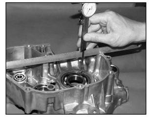
4. Measure the distance from the Magneto crankcase mating surface to the main bearing using the same method and record.
