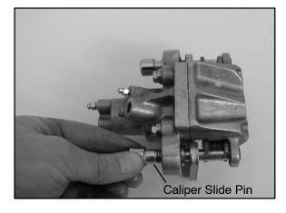
Caliper Slide Pin Torque: 30-35 ft. lbs. (41 Nm-48 Nm)
