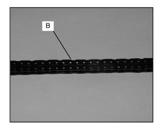
Remove cam chain (B). Inspect chain for worn or missing rollers or damage. Stretch chain tight on a flat surface and apply a 10 lb. (4.53 kg) load. Measure length of a 20 pitch section of chain. Replace if worn past service limit.
