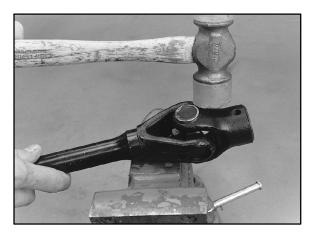
2. Support inner yoke as shown and drive outer yoke down (bearing cap out) with a soft face hammer.
