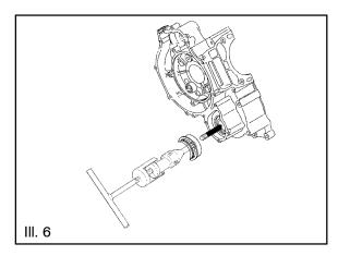
Turn the puller T-Handle clockwise until it contacts the water pump shaft. Continue rotating until the remaining portion of mechanical seal has been removed from the cases. Ill. 6 Pump shaft oil seal can also be replaced at this time if necessary. 7. The Water Pump Install Kit (**PN 5131135**) is required to install the new mechanical seal. This tool is available separately and it is also included in the Crankshaft/Water Pump Seal Installation Kit (**PN 2871283**).
